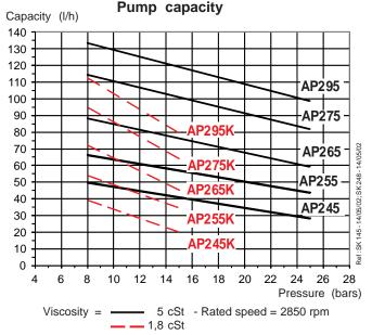
Data shown take into account a wear margin. Do not oversize the pump when selecting the gear capacity to ensure the optimum operation of the (NO) solenoid valve
