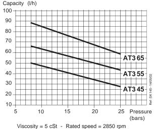
Data shown take into account a wear margin. Do not oversize the pump when selecting the gear capacity to ensure the optimum operation of the (NO) solenoid valve (switching low/high mode).
