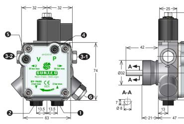
Inlet **1** and Return **2**with direct sealing
